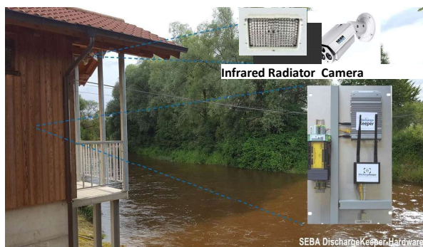
Figure 1: Hardware components of the DischargeKeeper for a typical measuring site
